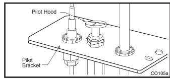
Fig. 9 Remove pilot hood.
